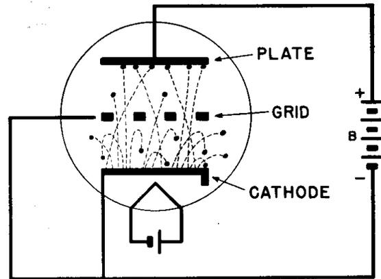
**FIGURE #9: With no grid bias there will be some number of electrons that will flow to the plate while the rest will form a space charge between the cathode and the grid.**
