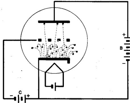
**Figure. #11. When you make the grid negative you will reduce the flow of electrons to the plate:**
