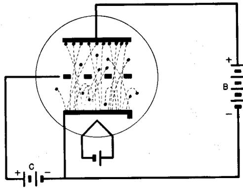
**Figure. 10: Making the grid positive with respect to the cathode will greatly increase the flow of electrons to the plate:**
