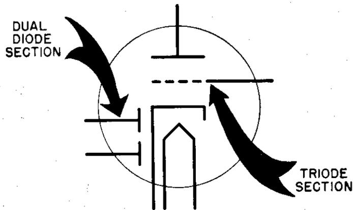
**Figure. #26. A combination tube containing two diodes and a triode. This is called a duo-diode triode.**
