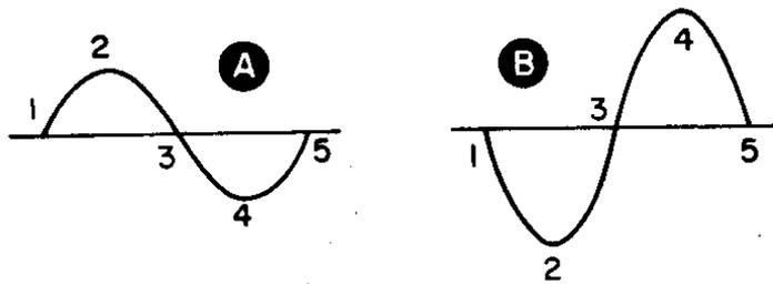
Figure. #14A & #14B. Figure "A" displays the sign wave signal voltage, while "B" represents the output signal voltage.
