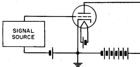
**Figure. #12. When a AC signal is applied between the grid and the cathode the result in an AC plate current.**
