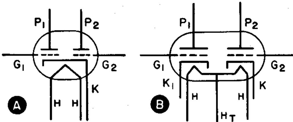
**Figure. #27. Dual triode tubes. The tube at “A” has a common cathode. The tube at “B” has two separate cathodes. Notice this tube has a single heater with a center tap. Not all tubes of this type have tapped heaters.**
