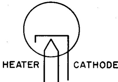
**FIGURE #3: Indirectly heated cathode symbol:**
