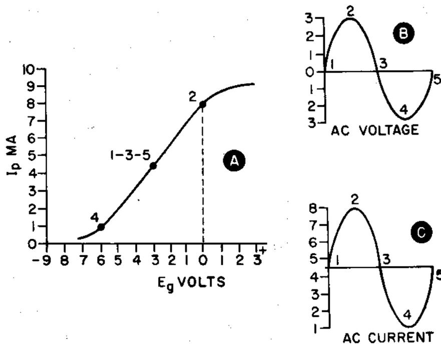
Figure. #17A & B & C. Figure "A" Is a typical characteristic curve, showing how the grid voltage "B" and the plate current "C" vary on it.
