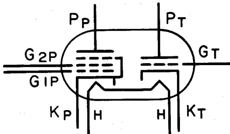
**Figure. #28. A pentode-triode combination.**
