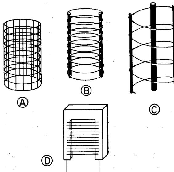
**FIGURE #8: Typical Grid Structures:**
