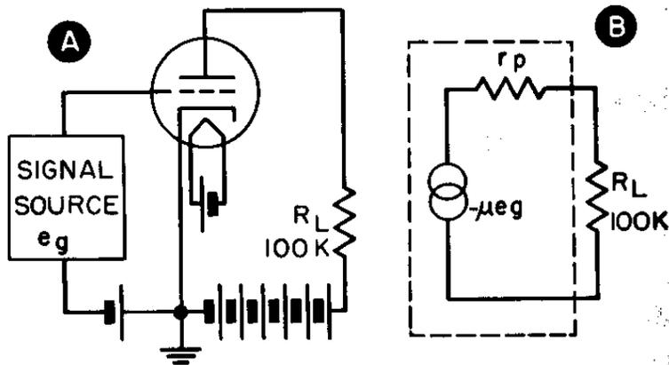
**Figure. #21. Simple amplifier circuit shown in figure “A” , and the equivalent circuit in “B”.**
