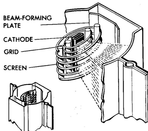
**Figure. #25. A beam-power tube structure:**
