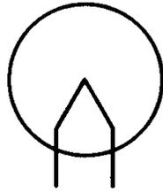
**FIGURE #1: Filament type Cathode:**
