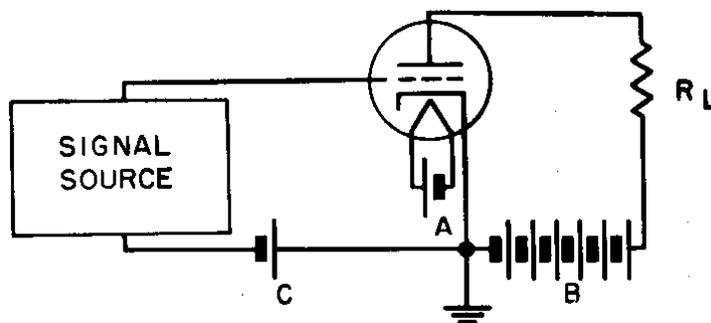
**Figure. #13. With a signal applied to the grid input you will develop a output signal across the plate load resistance from the plate current flow.**
