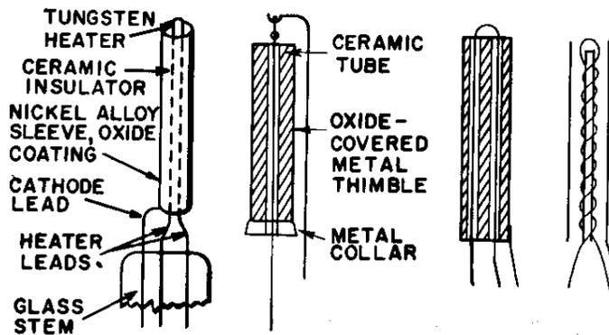
**FIGURE #4: Cathode Structure:**
