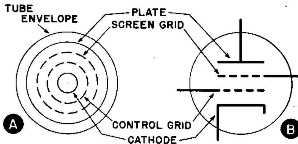
**Figure. #22. Figure "A" is of a Screen-grid tube cross section showing the arrangement of the elements; while figure "B", represents the schematic symbol.**
