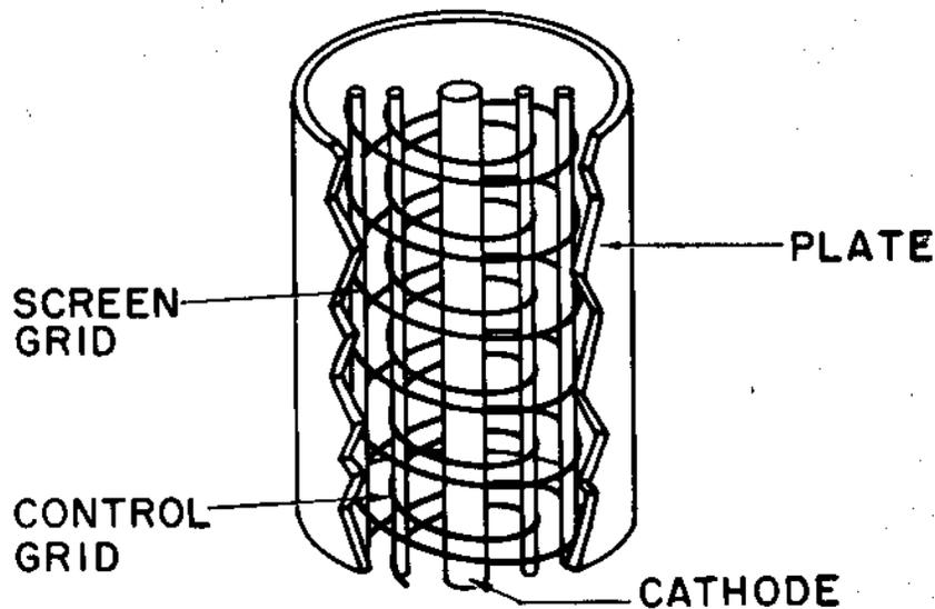
**Figure. #23 Cross section of Screen grid tube.**
