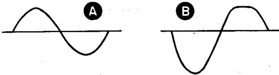
**Figure. #16 A/B: Input voltage = "A" and output voltage = "B" The flattened top on the right side of the "B" waveform is distortion from access bias:**
