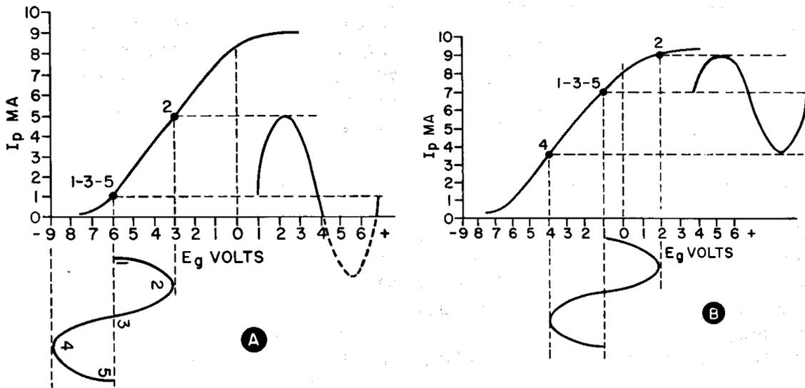
Figure. #19A and #19B: Figure "A" displays too much bias and "B" represents too little bias.
