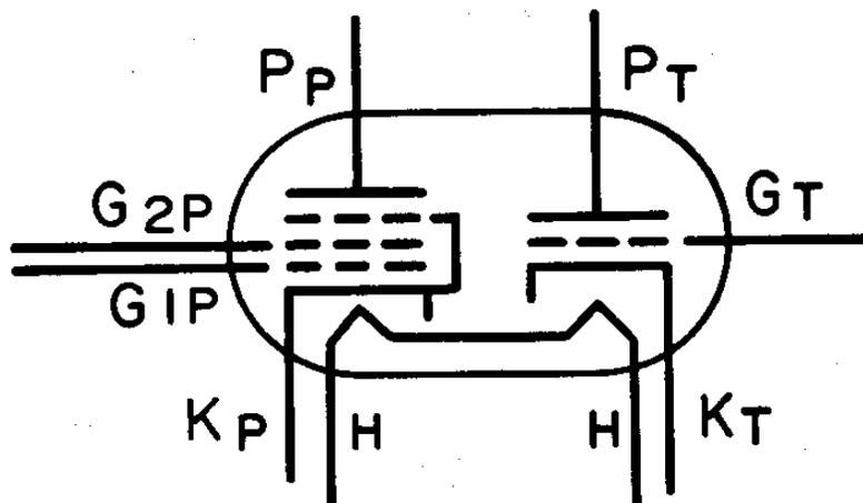
**Figure. #28. A pentode-triode combination.**
